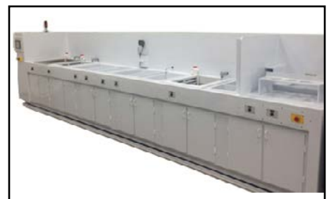
Passivation Wet Benches
